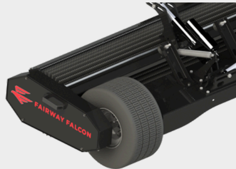
4. TURF TIRES 18" TURF TIRES USED TO REDUCE COMPACTION
